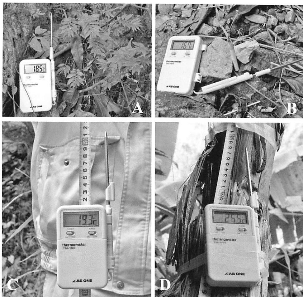
Fig. 6. Measurements of temperature at the wind caves. A: Near the ground at the wind cave in Xialai (site 11), 18.5 °C. (17:00, February 24th, 2010). B~C: Differences in temperature by height at the wind cave in a gully in Longmai (site 13). The temperature stood at 16.7 °C at the ground (B), 19.3 °C at 150 cm height, 25.5 °C at 230 cm height, respectively. (14:40~14:50, February 25th, 2010).
